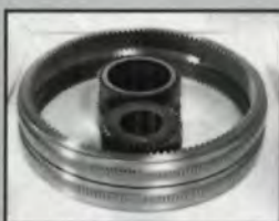
Fig. 1 — Planetary gear set, ground from the solid, using non-dressable CBN plated wheels.
