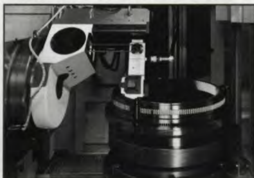
Fig. 2 — Pfauter CNC profile grinding machine with internal grinding arm and 58 mm diameter CBN-plated grinding wheel for grinding 117-tooth, internal double helical gear described in Fig. 1.
