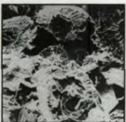
Fig. 13 — Magnified view of chips produced by CBN micromachining. Photo courtesy of Kapp.
