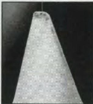
Fig. 4 — Phoenix 450HC-DRY with aerodynamic chip channel.
