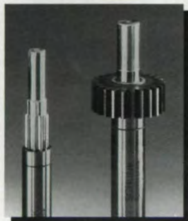
Hydraulic Arbor with and without gear.
