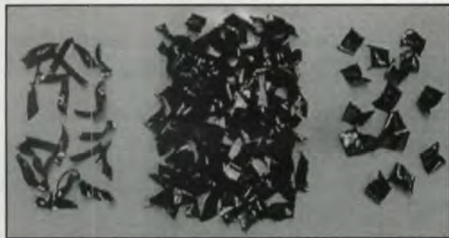
Fig. 3 — Chips from dry cutting; plunging on the left, roughing in center, finishing to the right.
