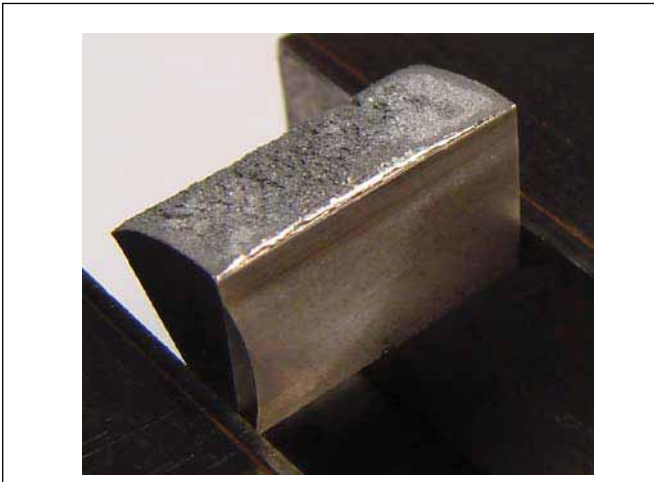
Figure 14 (a)—Wrought steel gear tooth impact fracture surface.
