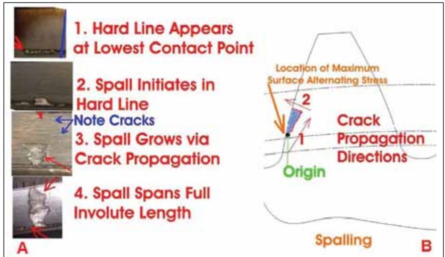
Figure 13—Initiation of a spall in a line of micropitting (the “hard line”).
