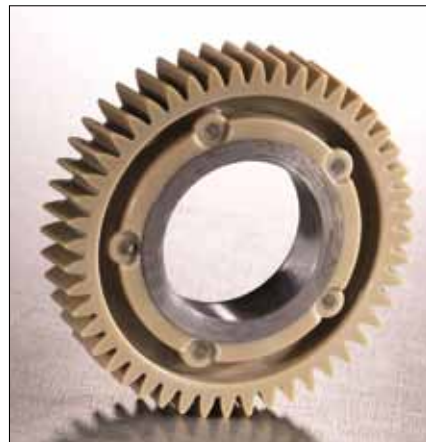
By switching from iron gears to PEEK, Metaldyne achieves roughly a 70 percent reduction in mass and almost 80 percent reduction in inertia in its balance shaft modules.
