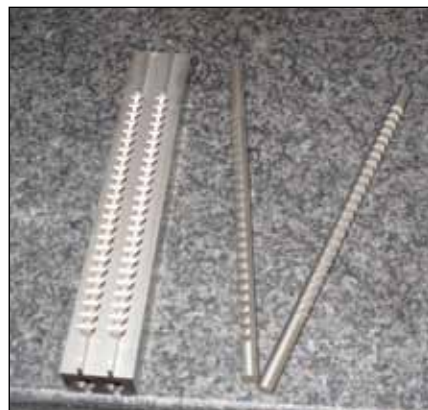
These broach tools were cut by MC Machinery on a wire EDM.
