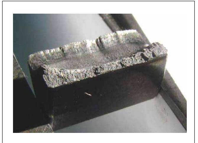
Figure 14 (b)—Ausform-finished P/F gear tooth impact fracture surface.
