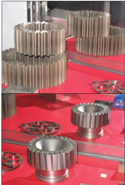
MC Machinery can cut basically any type of gear using wire EDM, except helical gears.
