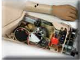
Articulating gear for the electric terminal device on the Utah Arm... patient can tie his shoes
