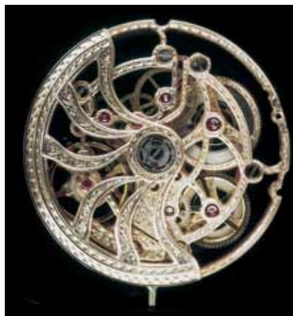
Wire EDM can be used for micro-machining applications, including the gears found in watches (courtesy of GF AgieCharmilles).
