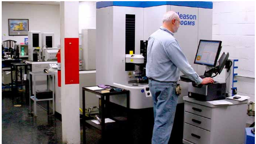
With installation of the next-generation Gleason 350GMS Analytical Gear Inspection System, Eaton Kings Mountain's gear lab is able to meet its high-volume gear and gear cutting tool inspection requirements: 1,500 parts per week, three shifts a day.
