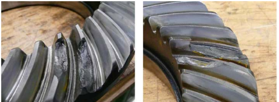
Figure 2 Flank breakage—two different wheels.
