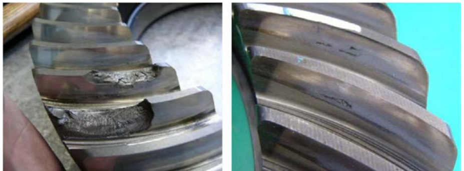
Figure 1 Flank breakage and pitting on wheel.
