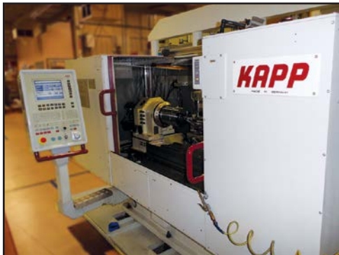
Gears for the Curiosity Rover were ground using the KAPP VUS 55P.
