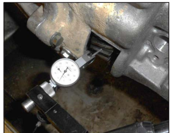
Figure 4 Backlash measurement of reverse idler gear.
