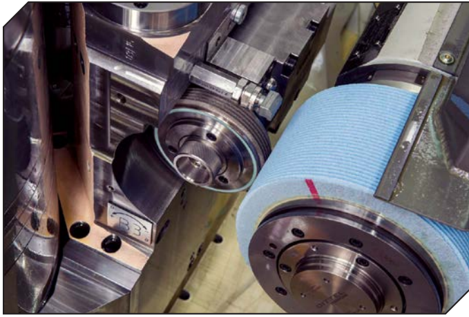
Figure 6 Multi-rib dressing of a sintered grinding worm saves time.
