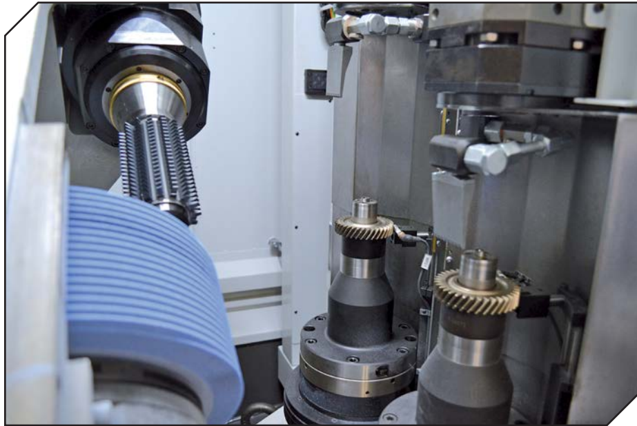
Double work spindles, driven by linear motors, make it possible to obtain a fast workpiece change and a chip-to-chip time under two seconds.
