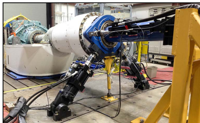
Figure 2 NREL 2.5 MW test stand with GB3 in background, and NTL hydraulic system in the foreground. The NTL system is used to impart non-torque loads into the hub flange of the test article, simulating wind turbine rotor hub loads.
