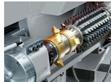
Chamfering in the work area
