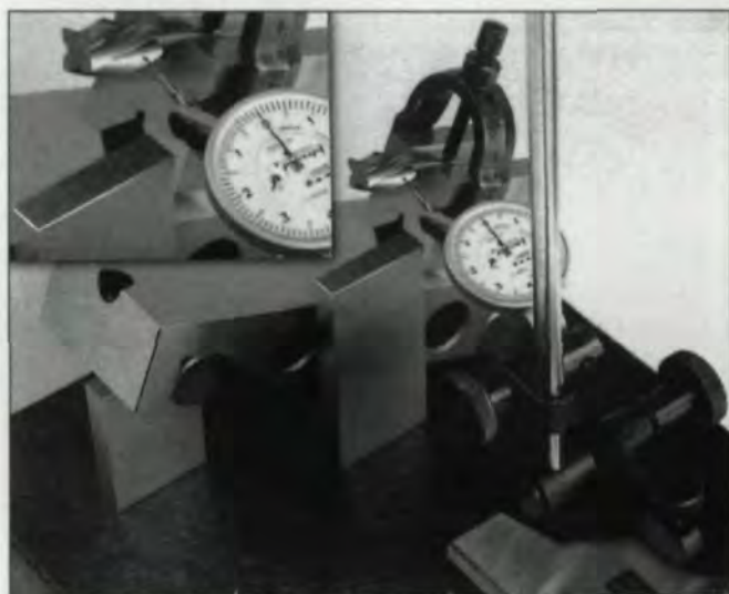
Sine bar setup for checking base helix error. Courtesy of Koro Industries Inc., Minneapolis, MN.
