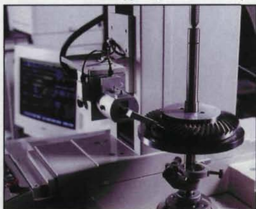
Figure 1—The scanning measuring method of hypoid gears.
