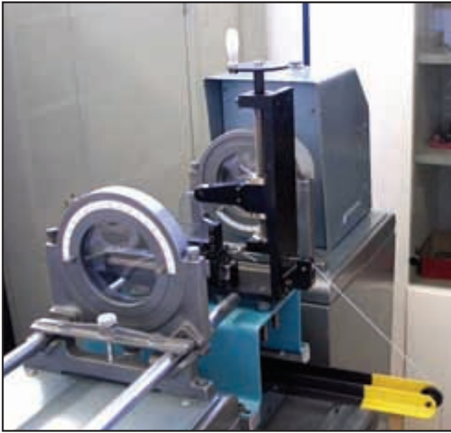
Figure 4—Test rig. Polarscope and loading apparatus with tooth specimen loaded at the tip.
