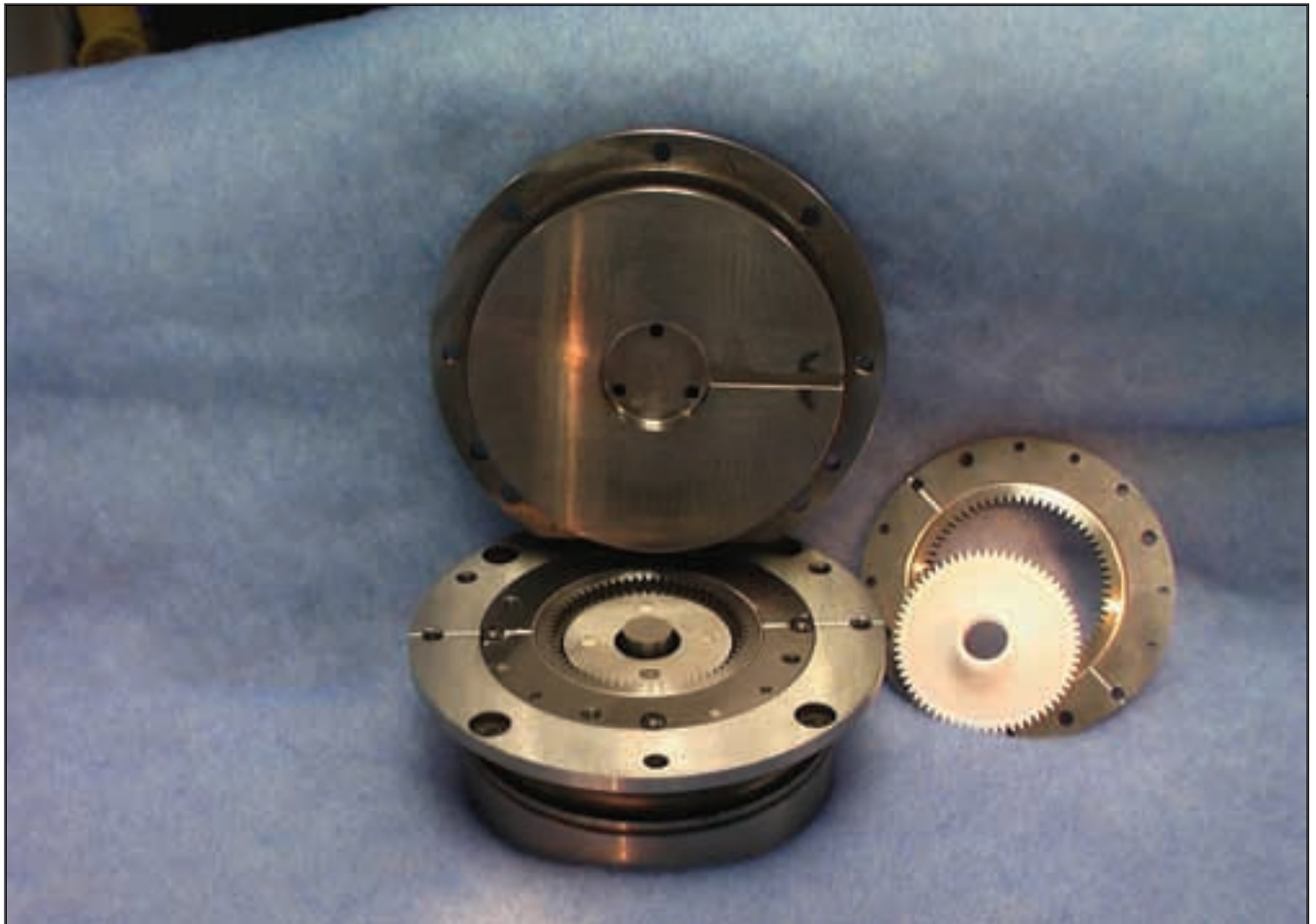
Figure 1—A molding insert tool alongside the molded gear and the gear cavity.
