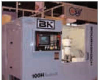
Bourn & Koch 100H CNC Horizontal Hobbing Machine – ideal for hobbing multiple splines and gears on shafts with tandem mounted hobs and milling cutters.
