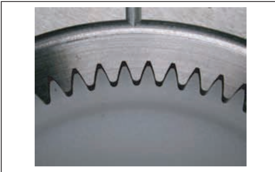
Figure 5—The involute shrinkage of a molded gear.
