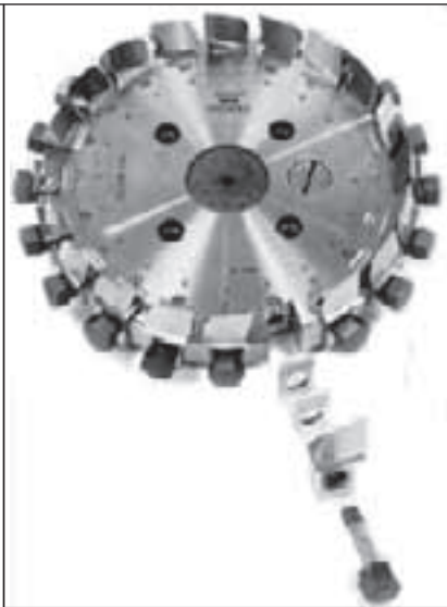
Figure 10—Face milled inserted blade cutter with parallel and shim used for mounting and truing blades on cutter head.
