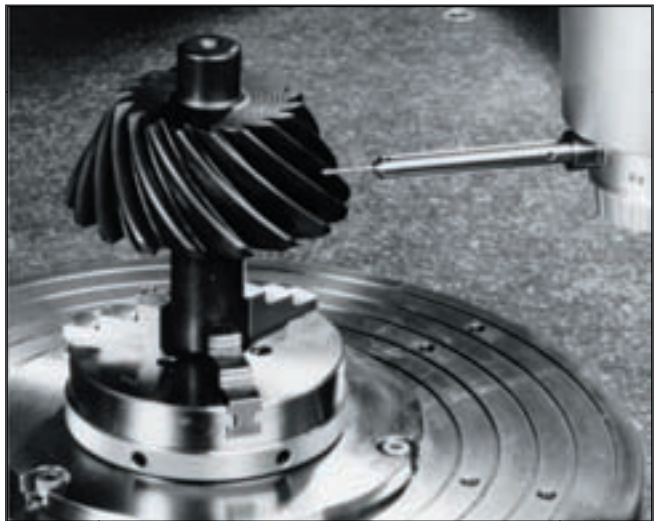
Figure 35—Close-up of a pinion being measured.
