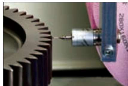
On-board inspection is one of many updated features of the Kapp KX500 Flex Gear Center.
