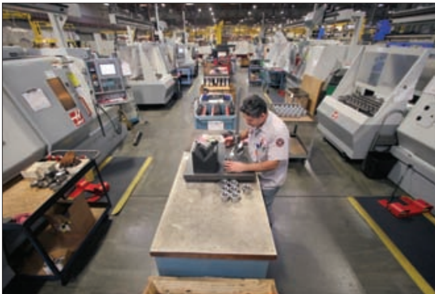
Haas lathes, with automatic parts loaders, can run unattended to reduce idle time.
