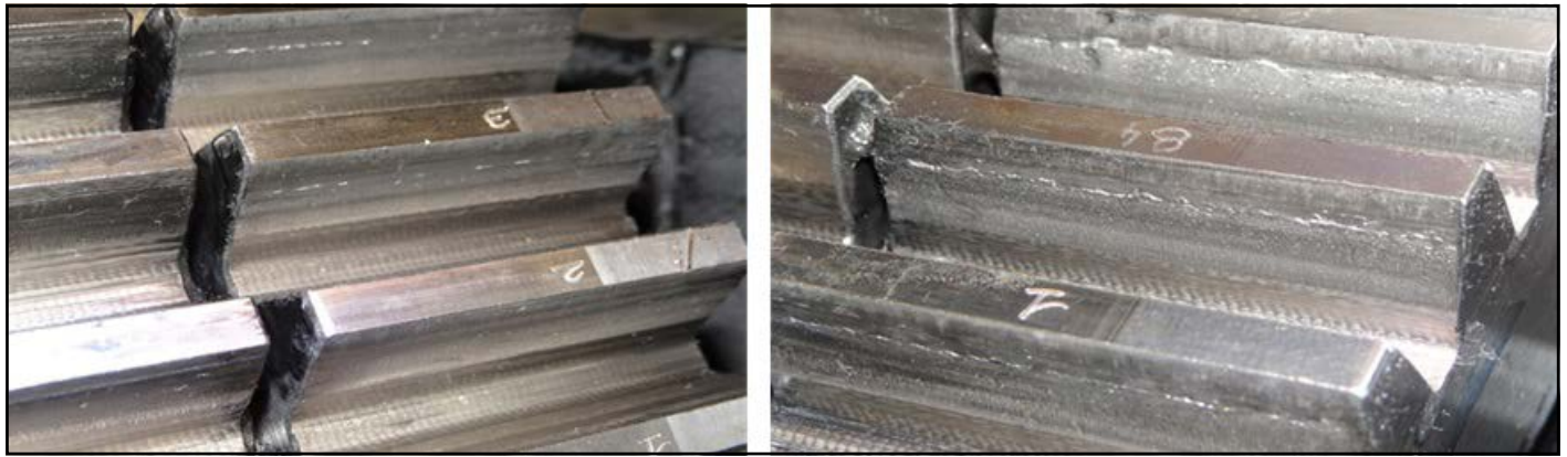
Figure 18 Tooth flank after 10 Mcycles at 1200 MPa.
