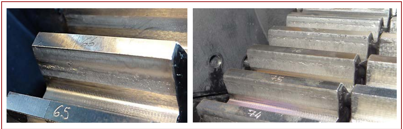
Figure 16 Tooth flank after 4.2 Mcycles at 1347 MPa (left) and 6 Mcycles at 1455 MPa (right).
