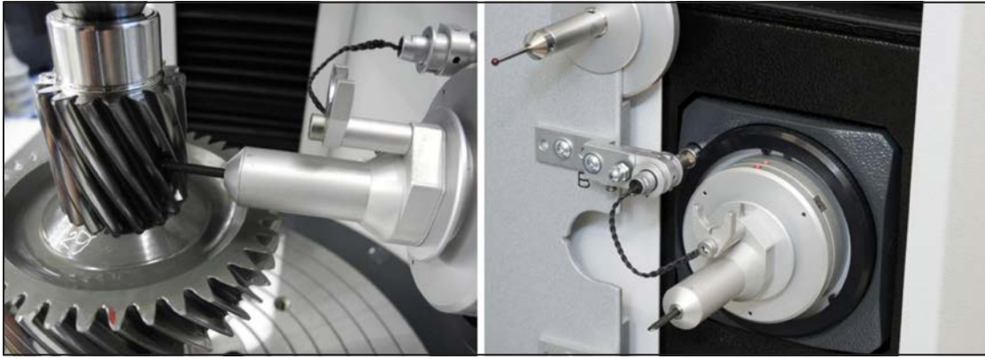
Figures 4 and 5 Roughness sensor mounted on the 3-D probe:
