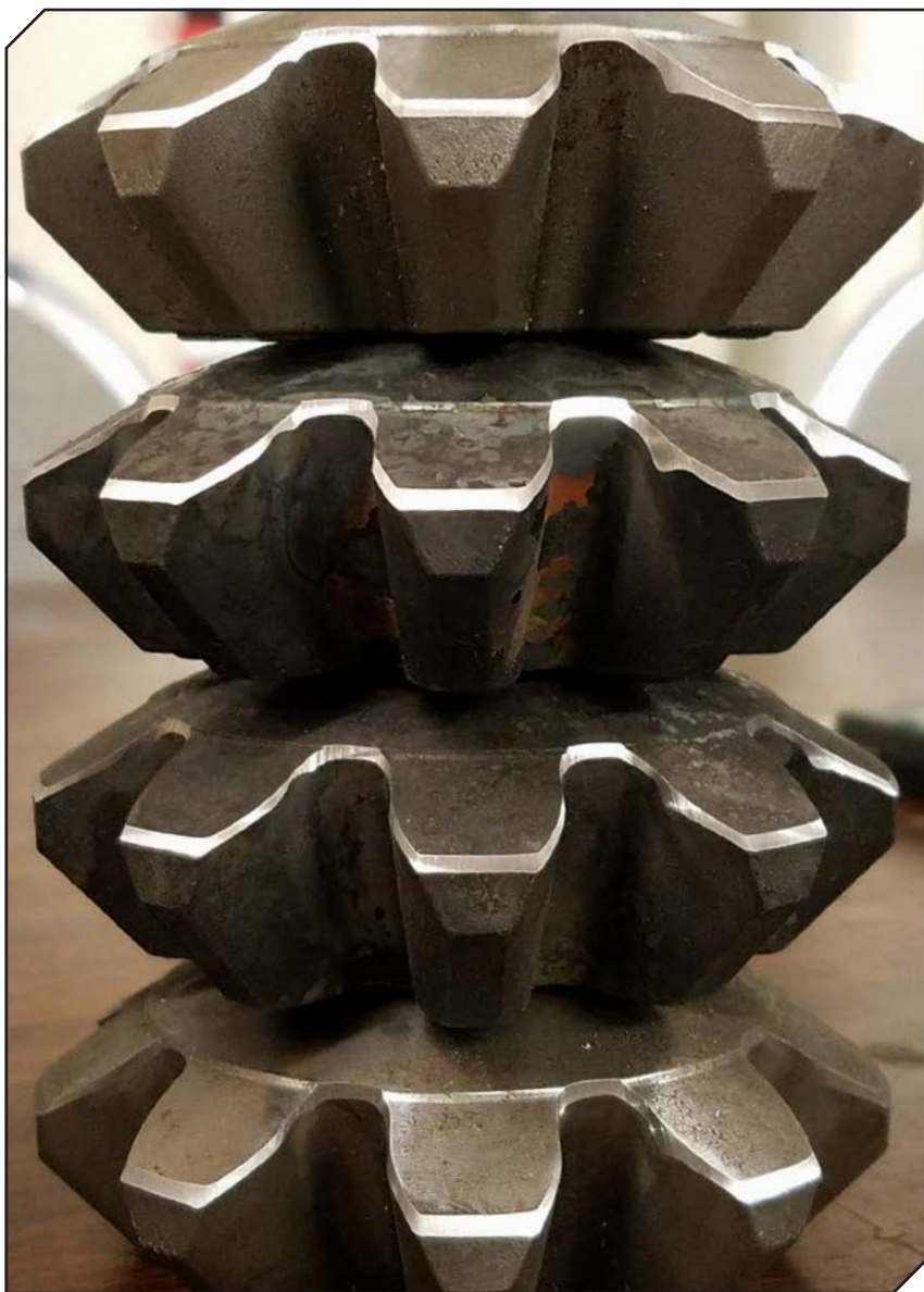
Figure 1 The four parts referenced in the article; No. 1, on bottom of stack, is the first soft part; No. 2, just above and on top of No. 1, is the first heat treated part after processing; No. 3 is next and on top of No. 2, and is the second heat treated part after processing; and No. 4 is the last soft part on top of No. 3, having been processed last. (Photo James Engineering).
