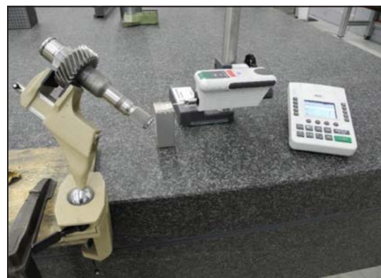
Figure 2 Reference plane scanning system.
