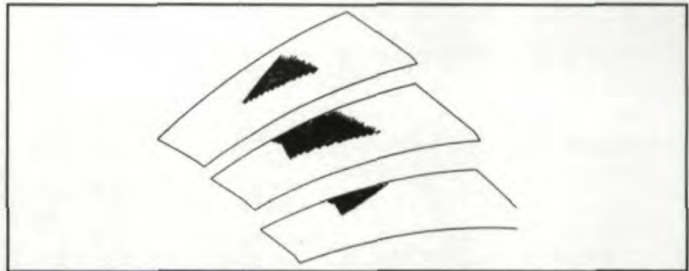
Fig. 18 — The locus of the contact zone at a gear torque of 960 in-lbs.
