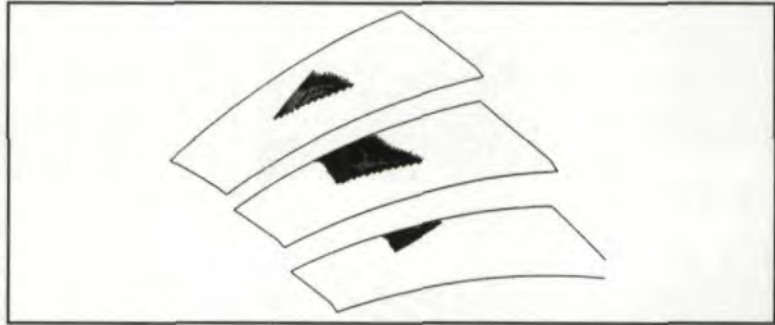
Fig. 17 — The locus of the contact zone at a gear torque of 480 in-lbs.
