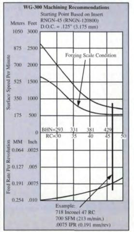
Fig. 5 - Sample nomogram for nickel alloy aircraft engines.
