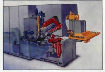
Fig. 1 — Concept hobbing machine for dry hobbing. Courtesy of Liebherr America. Used with permission.
