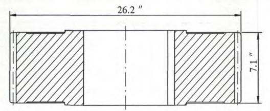
Gear for wind turbine drive system.
