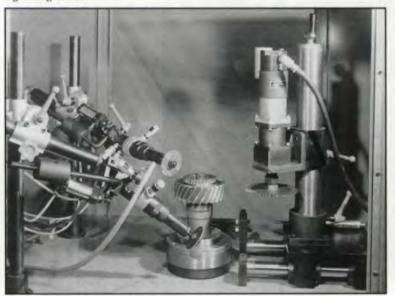
Fig. 3 — Removing exit burrs with a skiving unit and a grinding wheel. with the skive unit is started first. After the skived area rotates at least 45°, another workstation with either a grinding wheel or a brush mounted on it begins to work the skived area. As many workstations as required are energized accordingly. Thus at some point in time all stations are working simultaneously, cutting down on the overall cycle time.
