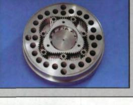
The complex geometry of the internal involute gear requires that the cutting tool will be mounted eccentrically and that a special back-off cam is available.
