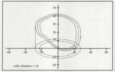
Fig. 1 - Three-dimensional track or cylindrical motion surface.
