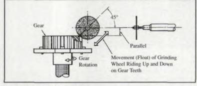
Fig. 4 - Alignment of grinding wheel.
