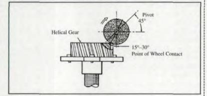
Fig. 6 - Helical gear wheel contact.
