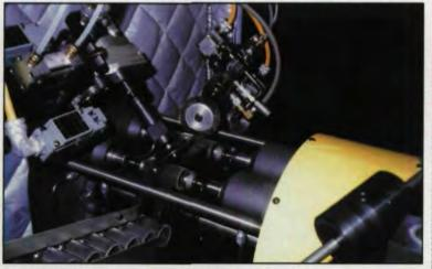
Fig. 1 — Deburring a helical pinion gear with power brushes. 26 GEAR TECHNOLOGY
