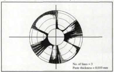
Fig. 4 — Bearing pattern for cylinder curve. facturing procedures results in high surface pressure and possible catastrophic part failure.
