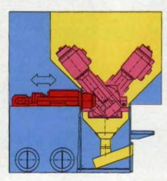
The entire work area is enclosed in a stainless steel shroud (yellow) that prevents hot chips from accumulating and directs them downward into a chip conveyor. Horizontal orientation of work spindle (red) helps facilitate chip removal.
