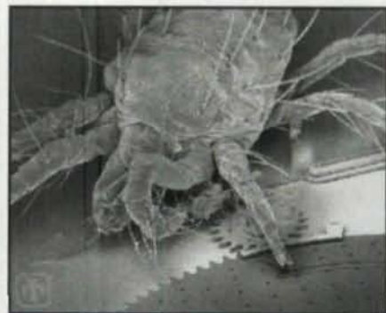
Fig. 5 — An electromicrograph showing a spider mite walking across microgears produced at Sandia National Laboratory.
