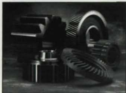
Fig. 4 — An assortment of gears forged by the Presrite Corporation.
