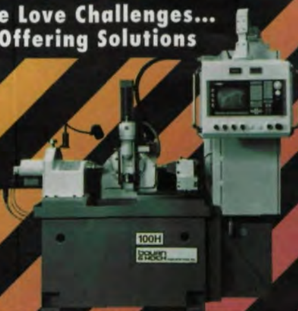
Standard Model 100H 4-axis hobber shown
