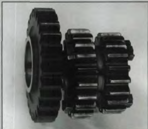
Gears from a racing motorcycle removed after an oil leak occurred during a race. The WC/C coated gear (on the left) shows very little wear, while the uncoated gears show severe adhesive wear. Courtesy of Balzers.
