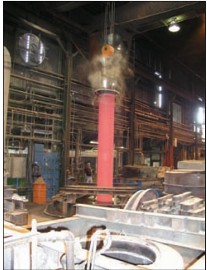
An in-process rope drum quenching at Xtek.
