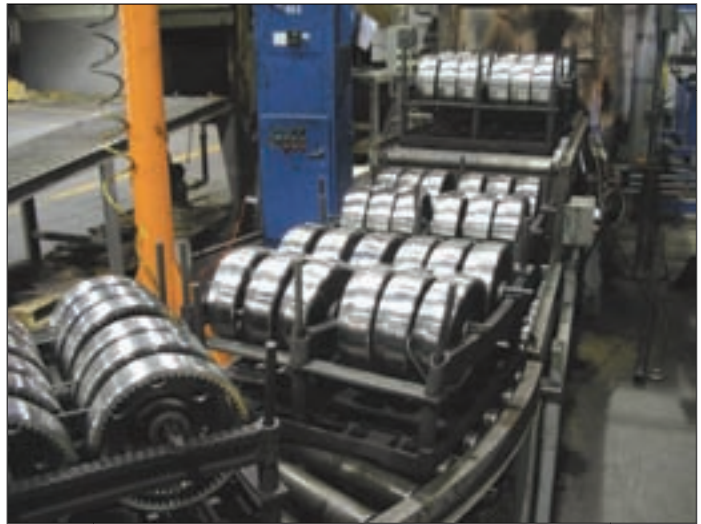
Closed-end gears fixtured for processing at Bodycote's New Berlin, WI. plant.
