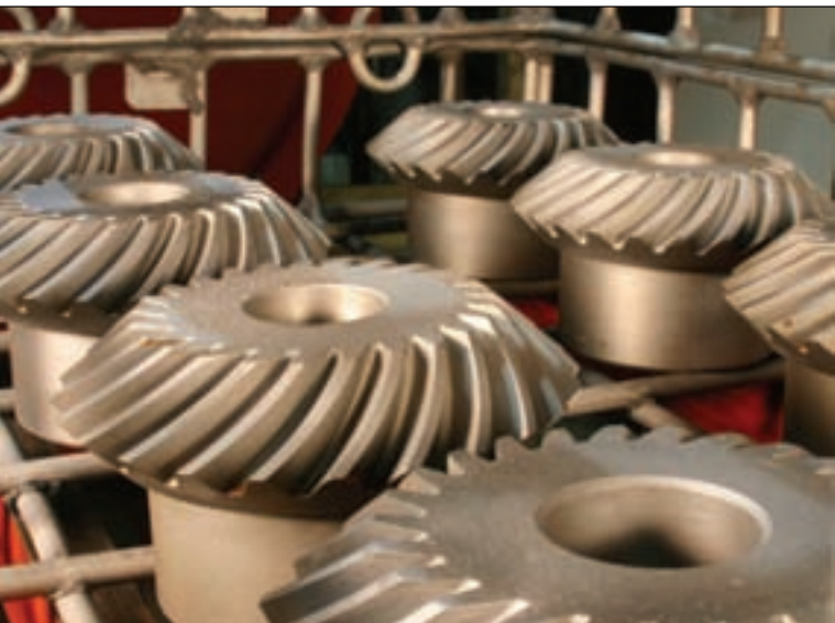
A tray of spiral bevel gears after vacuum carburization at Solar Atmospheres.
