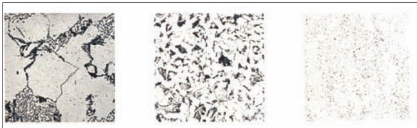
Figure 5—Steel structure of a forged blank (left), after normalizing (center) and after annealing (right).
