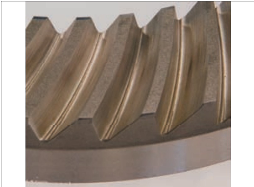
Figure 3—Unground root bottom in a ring gear.
