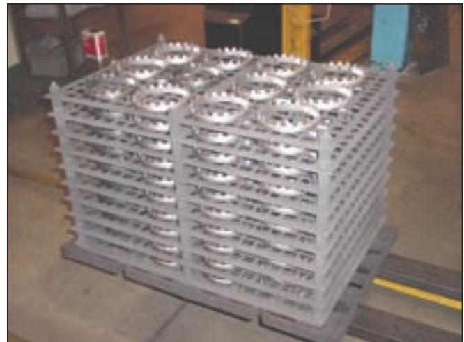
Figure 2—Load of internal rings on a graphite composite fixture.
