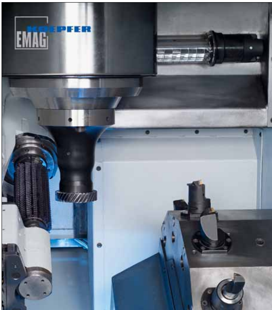
The EMAG/Koepfer twin-spindle VSC 400 DUO WF combines the functions of turning, gear hobbing, drilling and orientated milling on a single machine.
