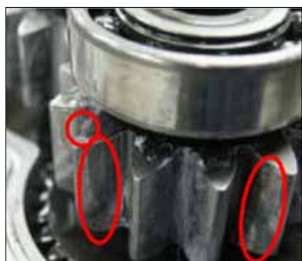
Figure 15—Damaged gear without crowning.
