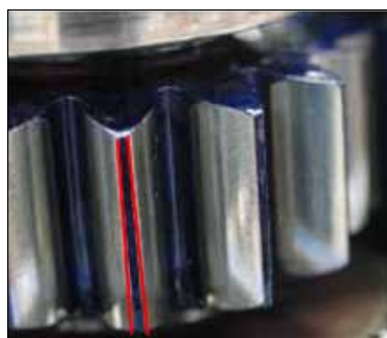
Figure 16—Good gear contact with crowning.
