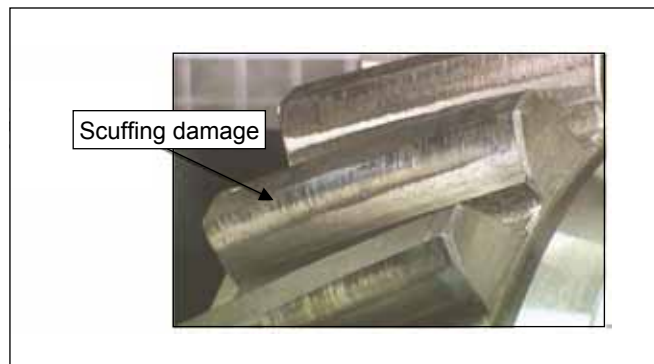
Figure 2—Scuffed gear sample from Design Unit's 160-mm center test rig.
