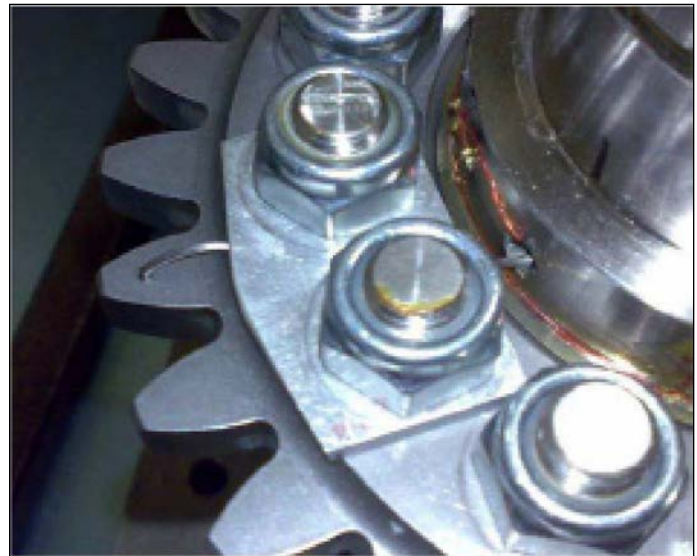
Figure 5 Gear equipped with thermocouple for bulk temperature measurement.
