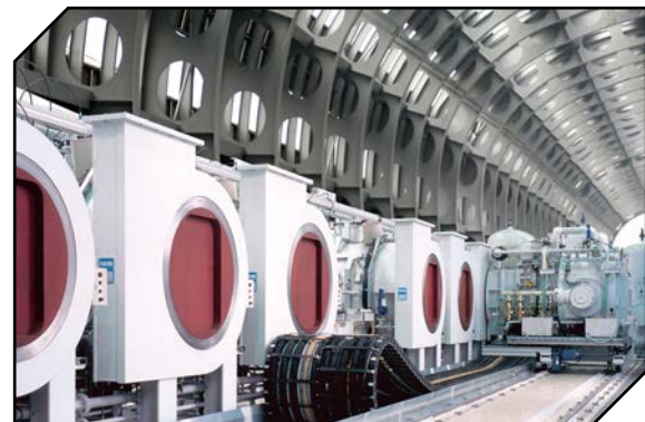
The latest technology in vacuum furnaces allows for ergonomic design and easy integration into the workflow of a manufacturing operation, as seen here with the ModulTherm concept from ALD-Holcroft. (courtesy ALD-Holcroft).
