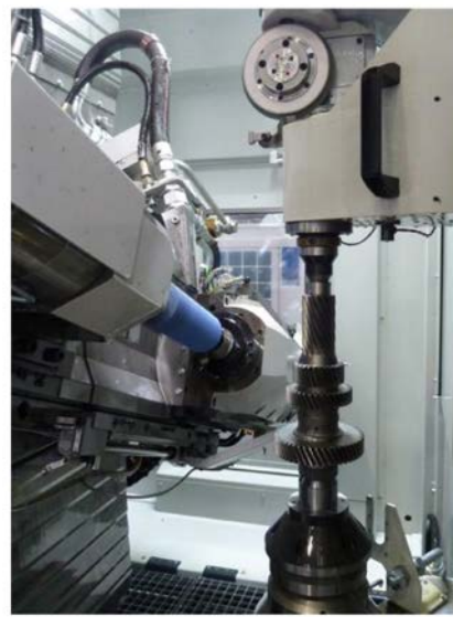
Figure 13 Drive shaft with asymmetric gear design.
