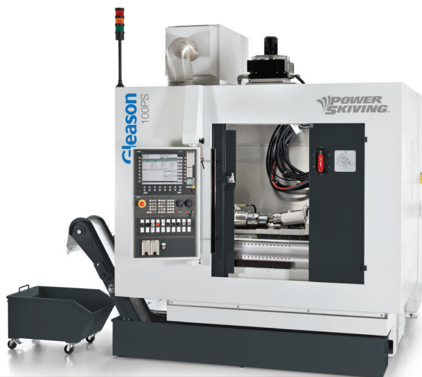
The Gleason 100PS power skiving machine offers small to medium-sized workpieces in module range up to 2.0 mm.
