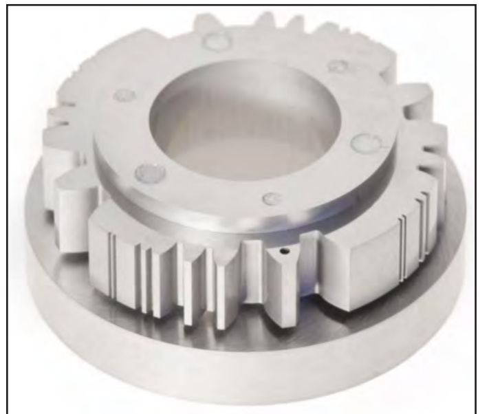
Figure 1 External microgear measurement standard. The bore hole denotes Tooth 1. The inner bore reduces the length to be penetrated by X-ray when measuring with the CT system.
