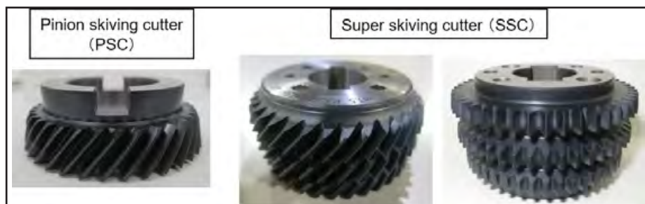
Figure 2 Appearance of pinion skiving cutter (PSC) and super skiving cutter (SSC).
