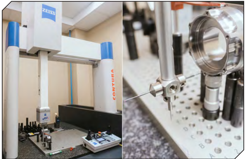
The facility has its own dedicated Zeiss Contura CMM, putting inspection in close proximity to the shop floor to reduce queue time.
