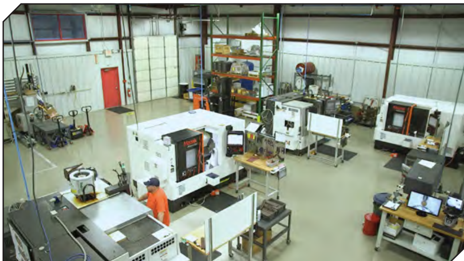
The 8,500 sq. ft. facility includes Mazak Quick Turn Turning Centers with multi-tasking capability so both turning and milling can be done in just one setup for shorter lead times and greater accuracy.
