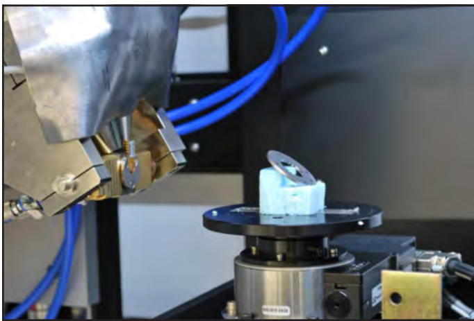
Figure 5 Measurement setup of the CT system. The X-ray source can be seen on the left-hand side of the image above. The measurement standard, positioned on the rotary table, can be seen on the right. The detector is situated on the far-right side and is not depicted in the image above.
