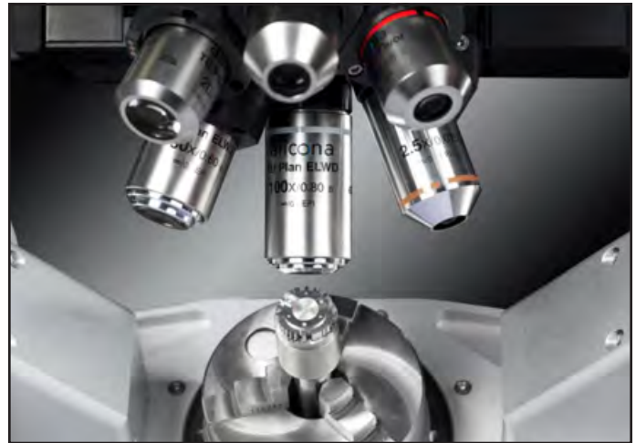
Figure 8 Measurement setup of the Alicona InfiniteFocus. The measuring machine allows roughness measurements and 3-D measurements to be performed.
