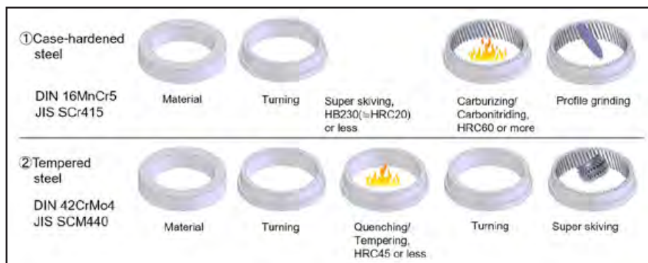
Figure 3 Manufacturing process of internal gear.
