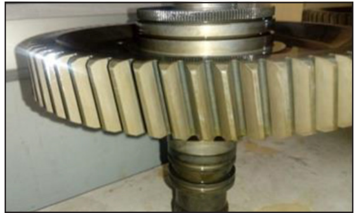
Figure 8b Image of gear flank after grinding burn test.
