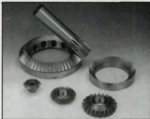
Figure 1—45°-shaft-angle crown gears and a 135°-shaft-angle crown gear for milling machines.
