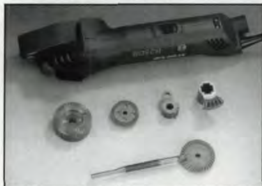
Figure 5—Sintered crown gears.
