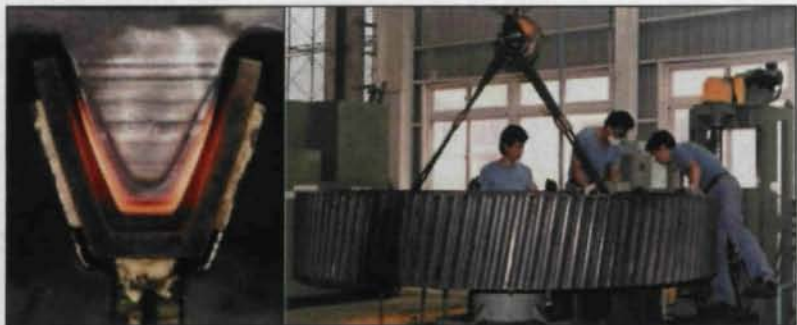
Figure 3—Induction hardening of tooth flank only. The gear has 92 teeth, each one 405 mm long, a module of 36.4, an outside diameter of 3,115 mm and is made of SCNCrM2A, a JIS material specification.
