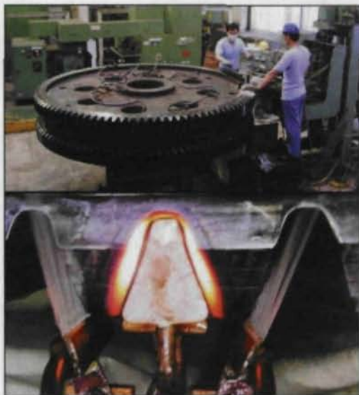
Figure 5—Induction hardening of tooth flank and root. The gear has 108 teeth, each one 182 mm long, a module of 25, an outside diameter of 2,776 mm and is made of SCM440, a JIS material specification.
