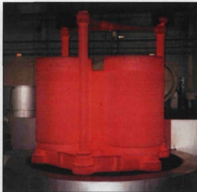
Figure 20—Arrangement of gears before carburizing in a new process furnace. Each load consists of 20 gears. Each gear has 107 teeth, each one 160 mm long, a module of 9, an outside diameter of 980 mm and is made of 17CrNiMo6, a DIN material specification. Case depth of gears is 2.8 mm.
