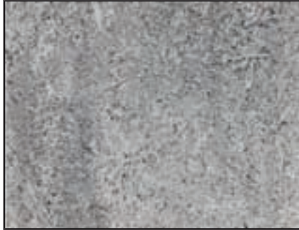
Figure 8—Sample C center microstructure 100X, 5% nital etch (Ref. 10).
