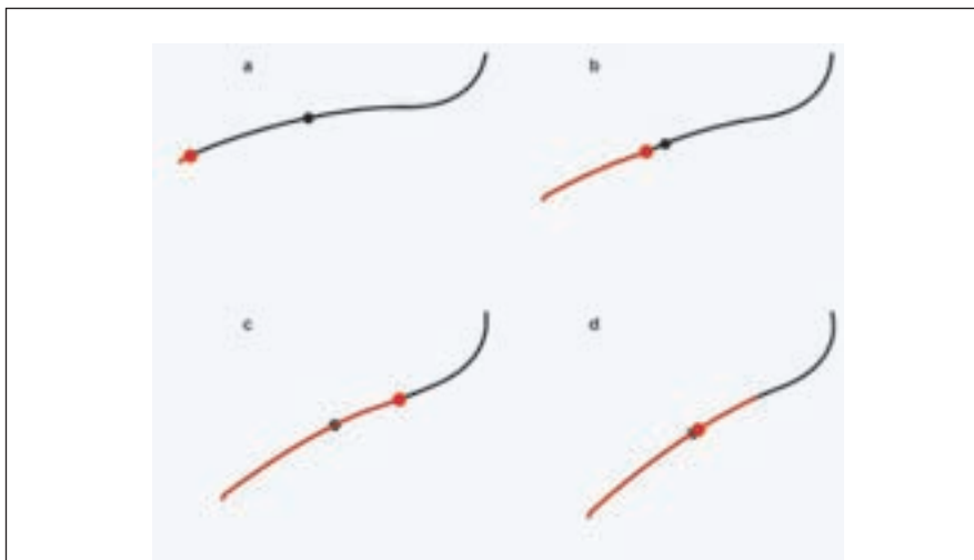
Figure 8—Kinematics of two meshing tooth flanks (only gear flank is drawn). The solid black line represents the tooth flank of the gear, the black dot represents the pitch point, the red dot represents the moving contact point and the solid red line represents the part of the flank that has already been in contact.
