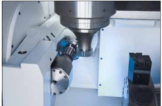
The VSC DUO WF from EMAG features both gear turning and gear hobbing operations.
