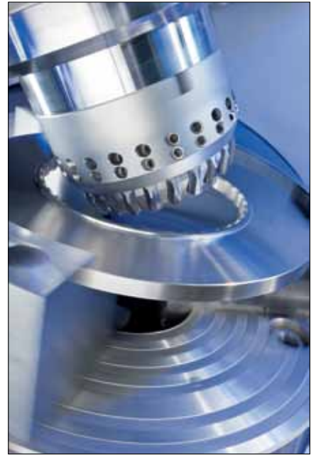
Skiving can be executed on the Oerlikon C29 and C50 bevel gear milling machines. These machines ensure a highly-precise coupling of all movements which are necessary for skiving.
