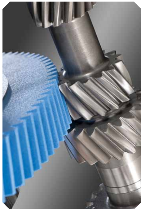
The Grono 250 uses an innovative gear honing wheel with external teeth.
