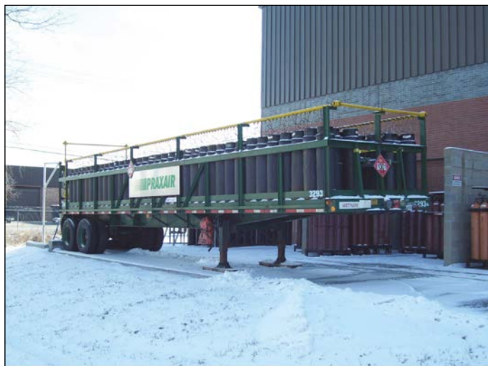
Figure 5 A typical trailer set-up: chemical acetylene with DMF solvent.
