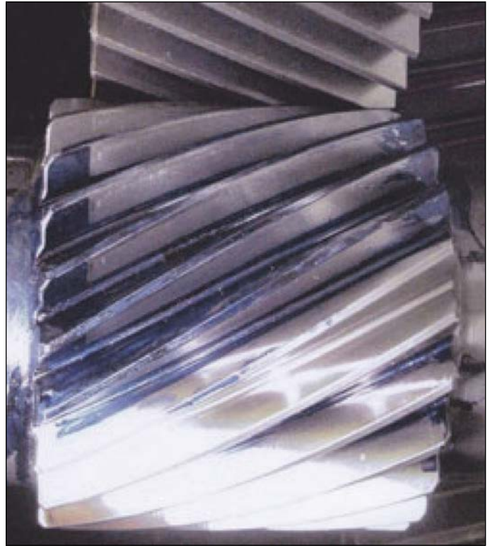
Figure 8 Pattern recorded at 100 percent load.
