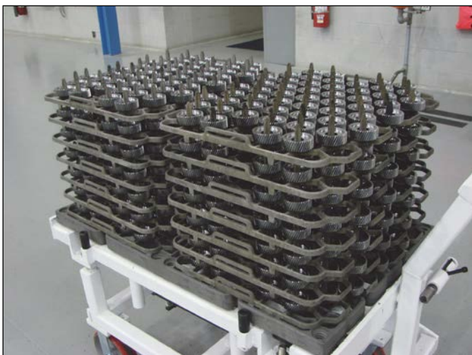
Figure 6 Load of input sun gears ready for processing.
