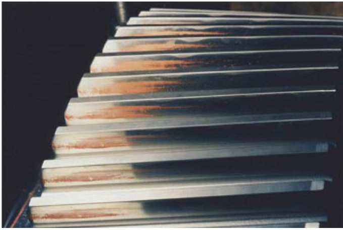
Figure 5 Different sector of unpainted gear revealed.
