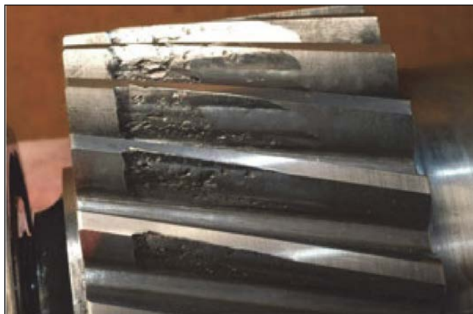
Figure 3 Severe misalignment can cause macropitting on helical pinion gears.
