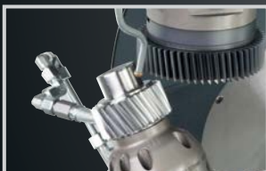
Power Skiving on a Bevel Gear Cutting Machine C 30
