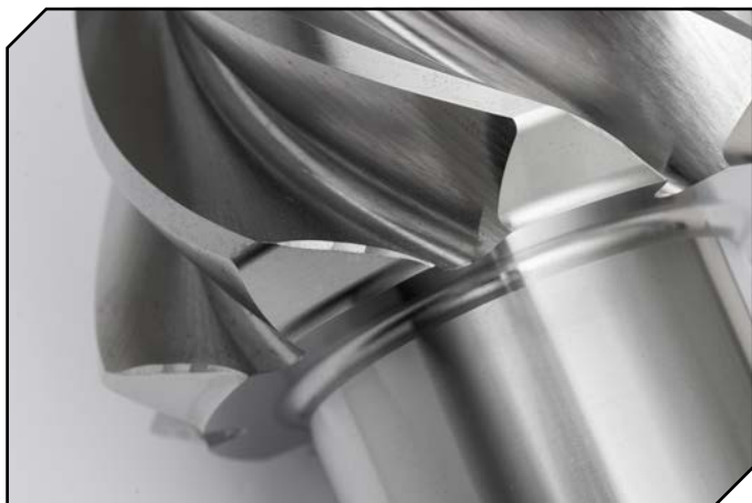
Figure 7 Contour generated with five different positions of the deburring tool.
