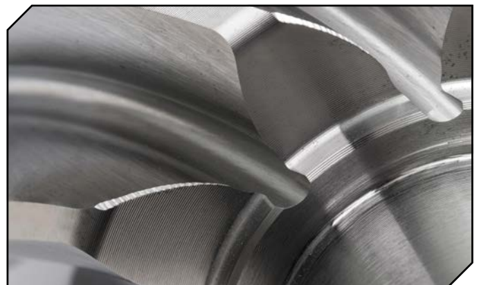
Figure 8 Contour generated with many different positions of the deburring tool.
