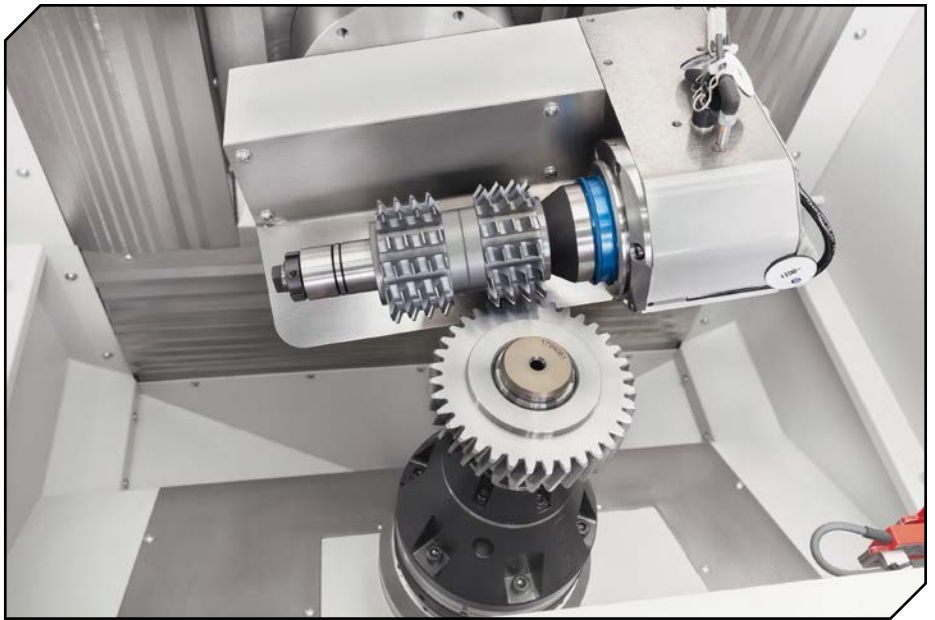
Two chamfer hobs for independent chamfering of left and right flanks.
