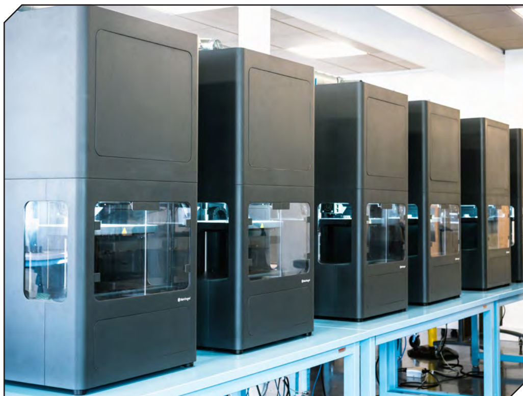
A Metal X Print Farm (courtesy of Markforged).
