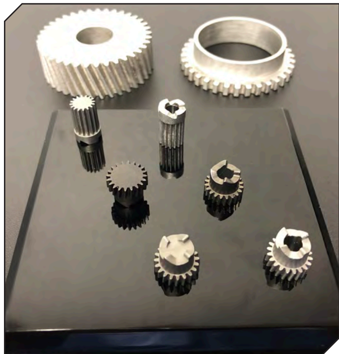
Metal 3-D printed gears from 3DEO.
