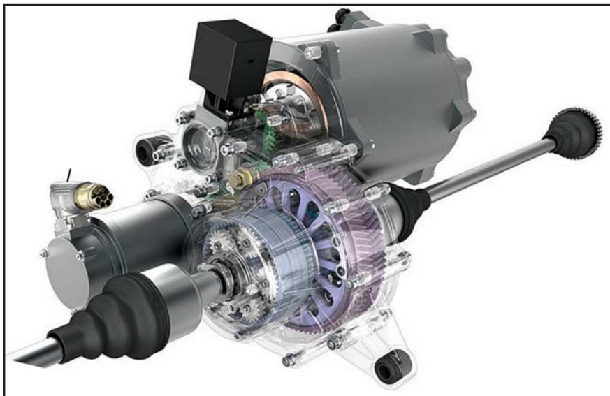
Figure 5 Three-stage variable ratio electric vehicle transmission — max ratio 18 (Ref. 4).
