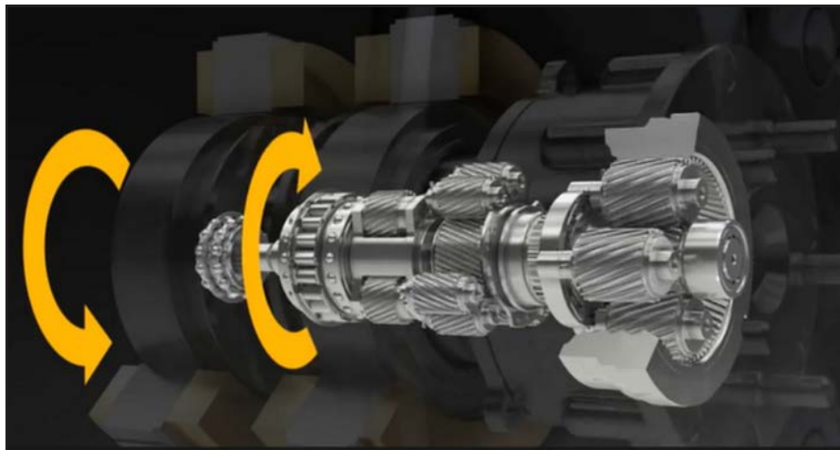
Figure 11 Double-wheel hub motor with transmission (Ref. 11).
