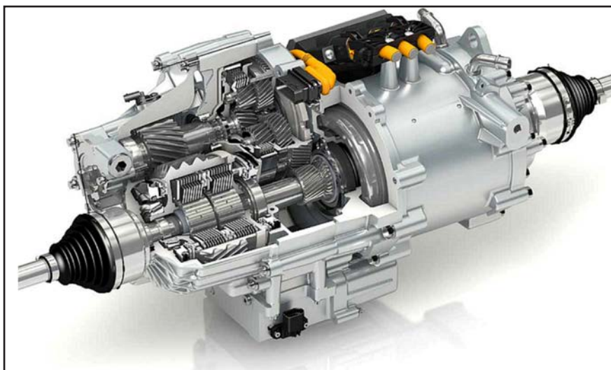
Figure 7 Four-stage and two-speed electric vehicle transmission — max ratio 20 (Ref. 6).
