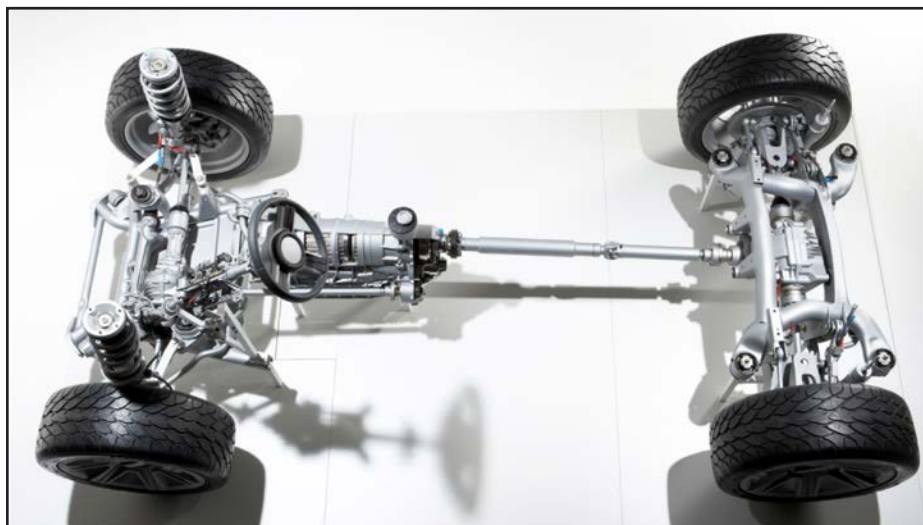
Figure 3 Powertrain in an all-wheel drive sedan (courtesy ZF Friedrichshafen AG).
