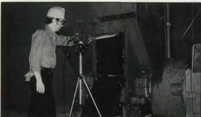
Fig. A-1—Test Set-Up Lens Type Infrared Radiation Thermometer
