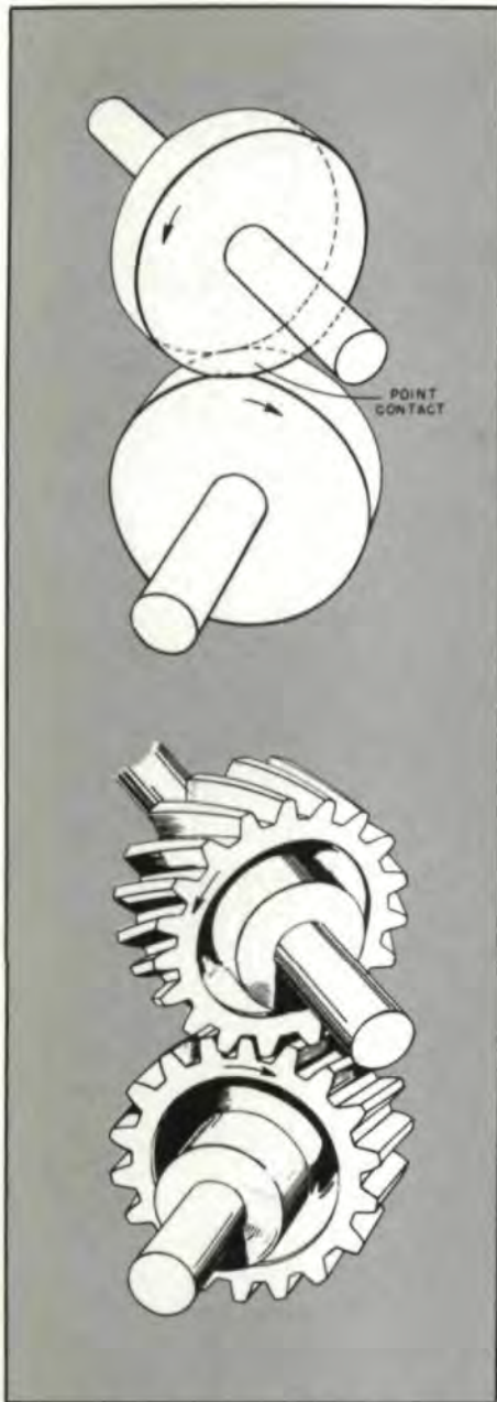
Fig. 7—Crossed helical gears. These gears transmit motion between nonintersecting shafts crossing at an acute angle. The teeth are developed on cylindrical pitch surfaces. Since only point contact exists between the gears, this arrangement is rarely used to transmit loads of any magnitude. (Courtesy of Mobil Oil Corporation.)
