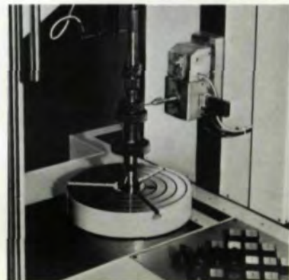
CNC controlled, 6 axis gear inspection machine
