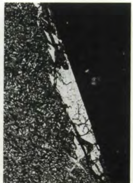
Fig. 6 – Position of the white etching areas in the area of the beginning of contact on the flank of the driving pinion.
