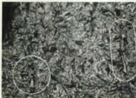
Fig. 4 – White etching areas at globular form sulfide inclusions beneath the flank surface.
