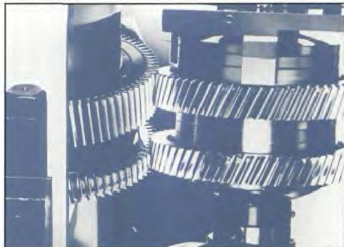
Fig. 6 — Mechanically constrained mesh of a CBN-coated tool with a crossed helical gearing.
