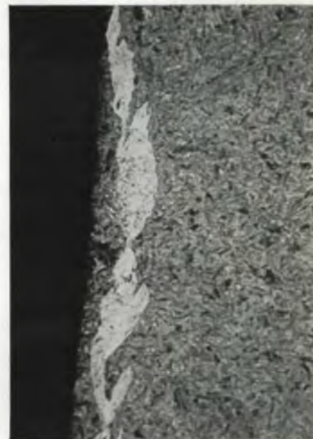
Fig. 15 - Flank damage on the pinion WEA at the surface in the area of initial pitting. ( P_c = 1560 \text{ N/mm}^2 ).
