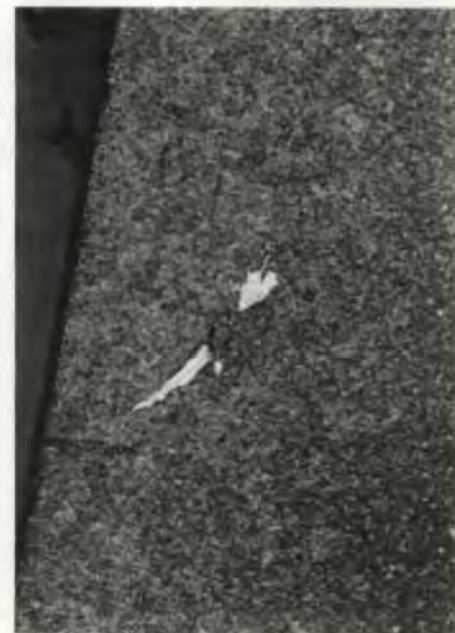
Fig. 3—WEA starting from an oxide inclusion beneath the flank surface of a case-hardened gear of 16 Mn Cr 5.
