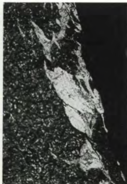
Fig. 7 – White etching areas in the area of the beginning of contact on the surface of a case-hardened pinion made of 16 Mn Cr 5.
