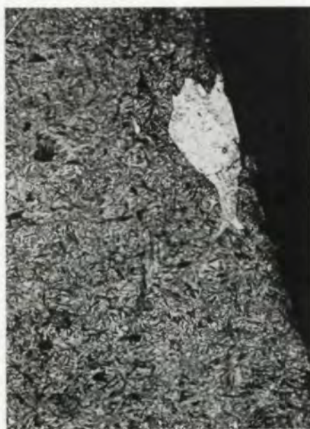
Fig. 14 - Flank damage on a pinion. WEA at the surface in the area of initial pitting ( P_c = 1600 \text{ N/mm}^2 ).
