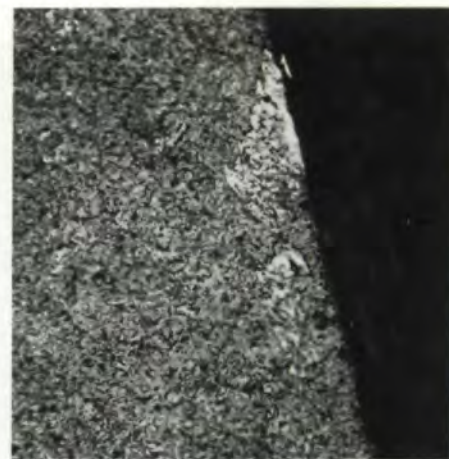
Fig. 12 – Partly tempered WEA at the flank surface.
