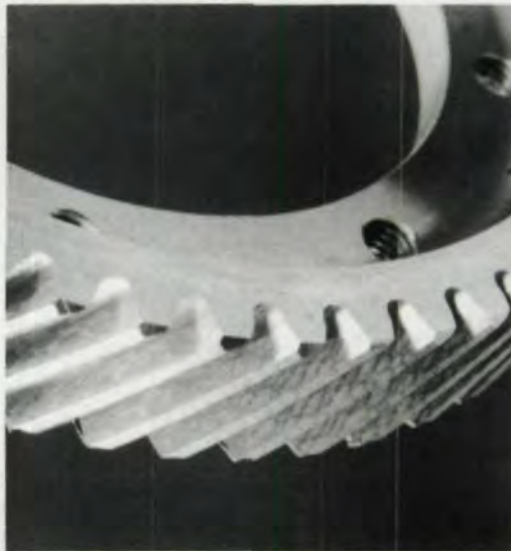
Fig. 2 - Gear tooth flanks produced by high feed rate, multi-thread hobbing.
