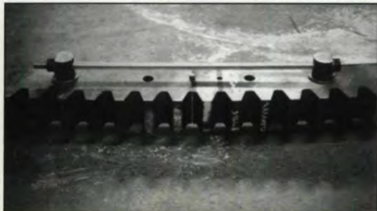
Fig. 1 — A close up view of the gear shows how the toothed sections were assembled during the roundup. Sections had to fit together with a very tight tolerance of \pm 5 mm on the 62' diameter.
