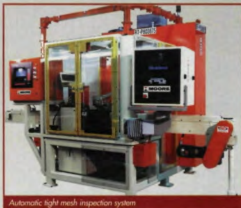
Automatic tight mesh inspection system
