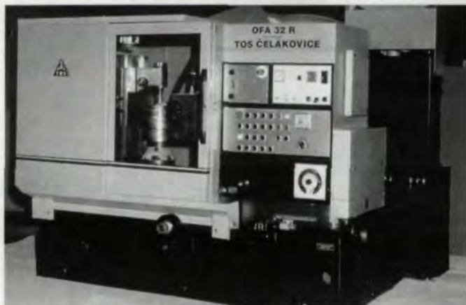
Gear Hobbing Machine, Model OFA 32 R
