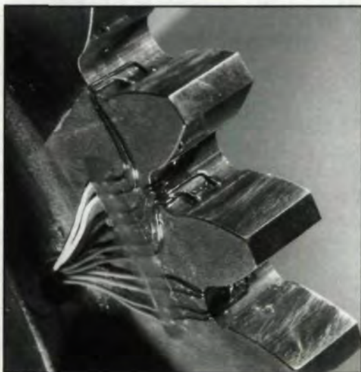
Fig. 2 — Strain gage installation on test gear.
