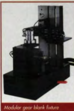
Modular gear blank fixture
