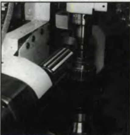
Close-up of gear being cut. All hobs are made of PM 45 high speed steel, TiN coated with AA tolerance. They have a single start and a class "AAA" line of action.
