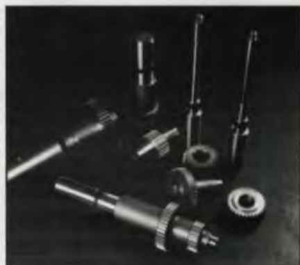
To streamline gear production at Ann Arbor Machine Co., most gears have the same pitch and pressure angles. Gears manufactured are usually straight spur gears and some with internal splines.
