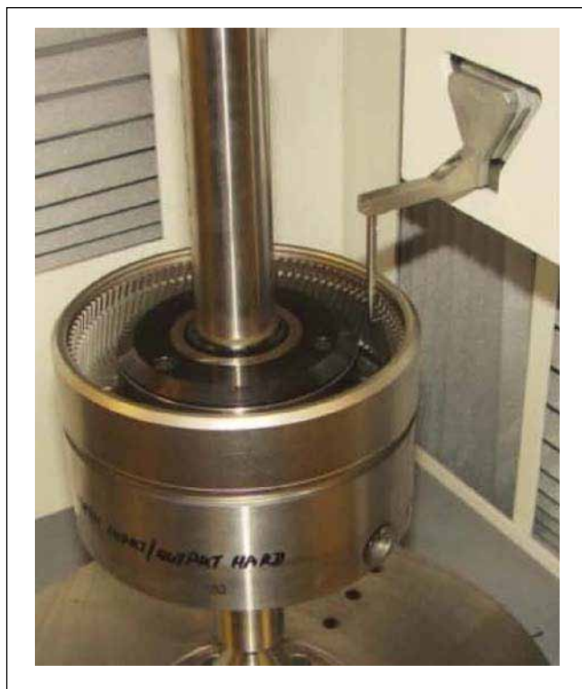
Figure 7—Geometrical inspection of an output internal gear with a CNC analytical gear checker.
