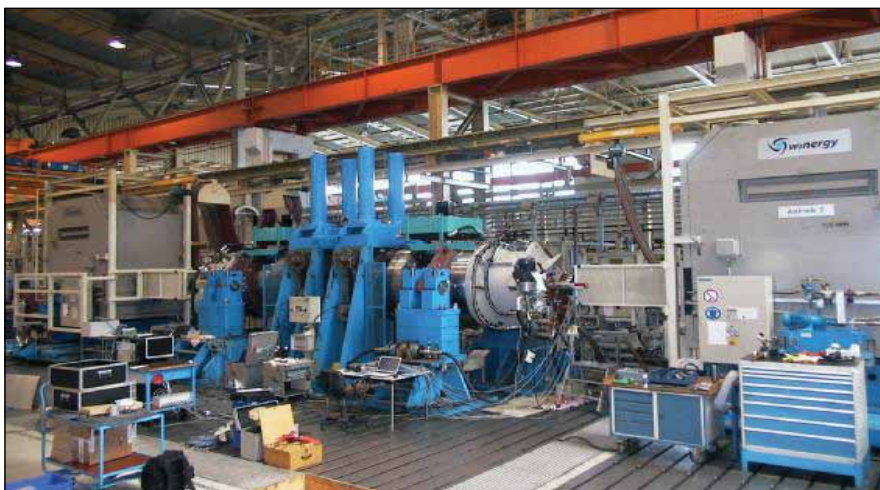
Figure 1—Back-to-back test rig at Winergy/Voerde during prototype test.
