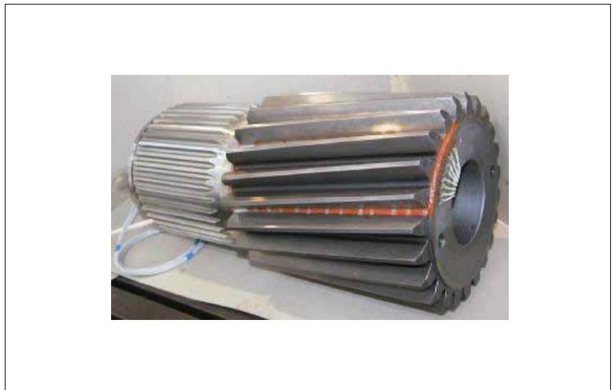
Figure 3—Application of strain gauges for load-distribution measurement on a sun pinion.
