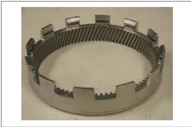
Figure 8—Input internal gear ( d = 139 mm, 89 internal teeth).
