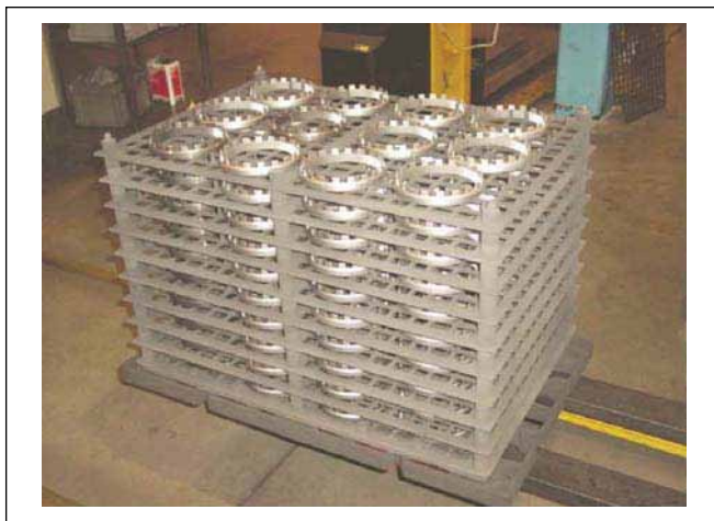
Figure 5—Load of internal ring gears on CFC fixturing.
