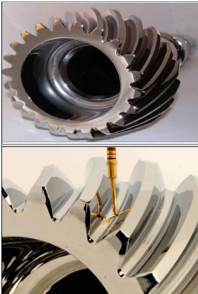
Figure 9 TTO bevel pinion post-MMP treatment.
