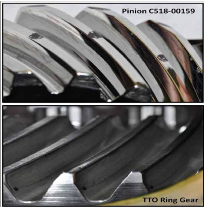
Figure 19 Post-test TTO pinion and bevel gear.
