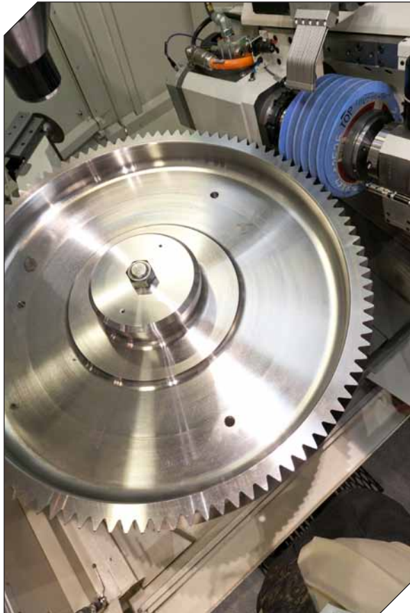
Kapp’s ZX 1000 features a large ductile iron bed and torque motor for high load capacity (photo by David Ropinski).
