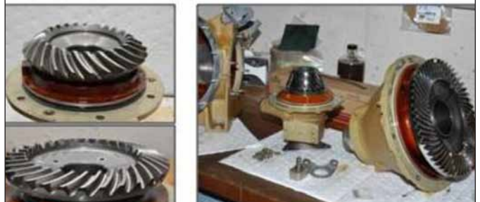
Figure 2 UH-60 tail drivetrain spiral bevel gears.
