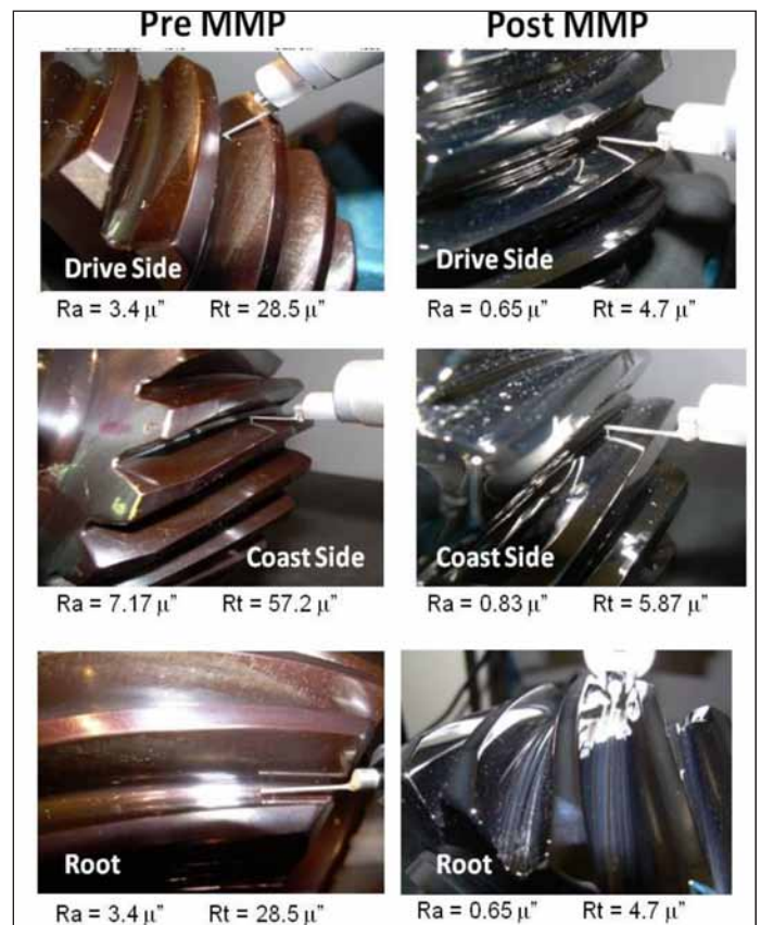
Figure 10 Pre- and post-MMP surface roughness of TTO bevel pinion C518-00159.
