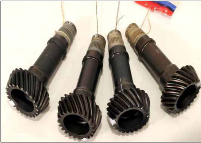
Figure 4 Candidate-TTO pinions as received from SAFR.
