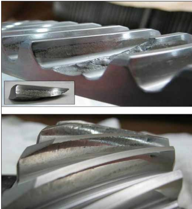
Figure 3 TTO bevel gear and pinion post-Block I overload testing.
