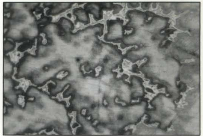
Fig. 8—Delta particles in dendritic alpha matrix tin bronze centrifugally cast-50x.
