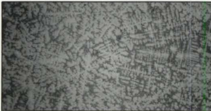
Fig. 7—Dendritic structure in alpha matrix tin bronze centrifugally cast-50x.
