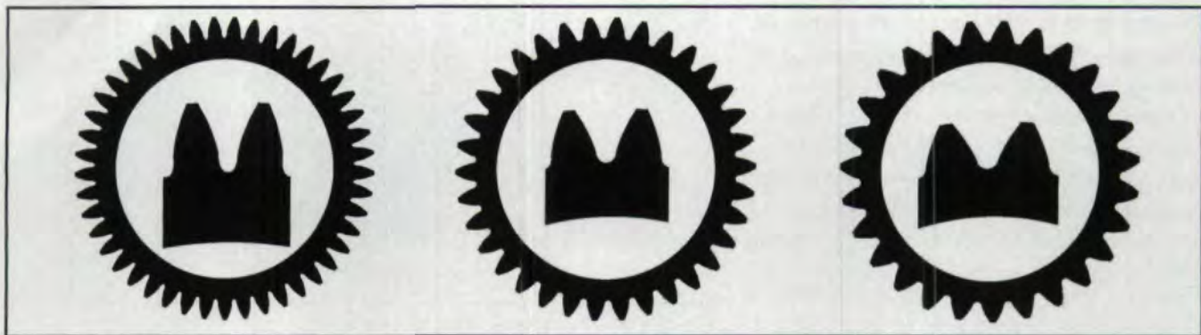
Fig. 5—The slender (left) and not-slender (right) geometry compared with the geometry of the original tooth (middle).
