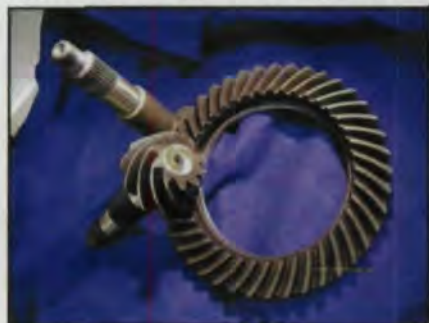
Laser peening is more effective than shot peening, and it's beginning to be used on gears, including this automotive ring and pinion set processed by LSP Technologies Inc.
