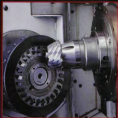
PENTAC™ Cutter System shown on new PHOENIX II 275HC Bevel Gear Cutting Machine.
