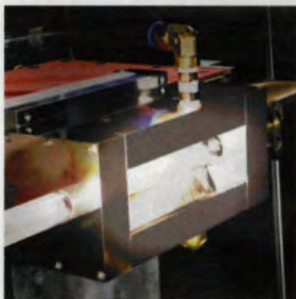
Capable of radiating 3.5 kW/cm 2 , Oak Ridge National Laboratory's plasma arc lamp glows brilliantly as it hardens steel without hardening the entire workpiece. The lamp's hardening ability could be used on internal gear teeth.
