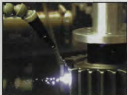
A pulsed laser beam creates a shock wave that causes beneficial compressive stresses in the roots of these gear teeth. Photo courtesy of Metal Improvement Co. Inc.
