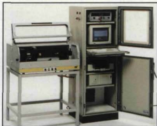
Figure 6—Gear inspection system, with gear inspection stand and computer/ROLLSCAN™ cabinet.
