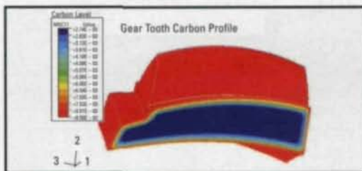
Figure 3—Carbon profile in carburized and quenched helical gear (units are weight fractions). us to focus on a single gear tooth, as shown in Figure 2. Cyclic symmetry conditions were applied to the cut faces of the model.
